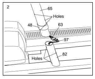
Slide the Upright Collar (48) to the position shown. Finger tighten three Upright Bolts (47) with Upright Washers (115) into the Upright (65). Note: It may be necessary to move the Upright slightly to align the holes.
